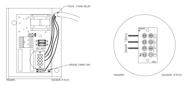
The neutral will only be used on 4-wire service. This is typical for 380-416V, 50 Hz.
